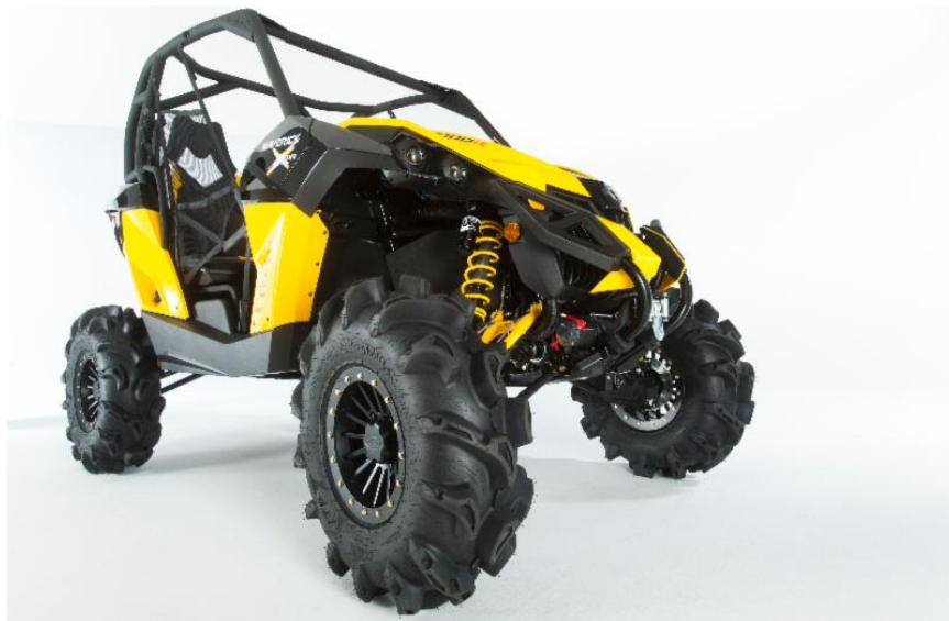
ITP SD Dual Beadlock Black Ops wheels featuring 32-inch ITP Monster Mayhem tires.
