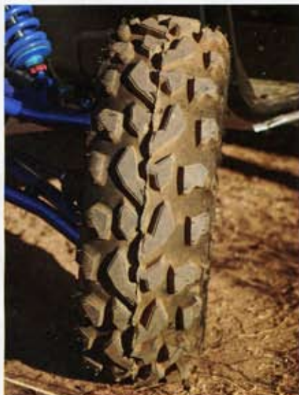
As you can see here, the BajaCross has an overlapping center lug pattern that makes for a smooth, tractable ride on hardpack. The side lugs work wonders in sand and rocks.
