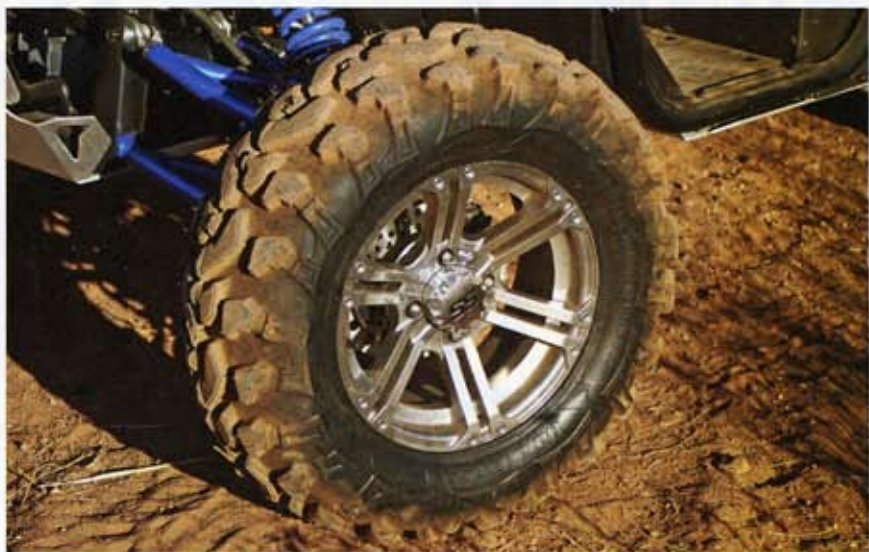
We had our BajaCross tires mounted on beautiful ITP SS212 Platinum wheel for extra bling points. The 14-inch wheels provide a mean look while reducing sidewall flex over a 12-inch wheel.
