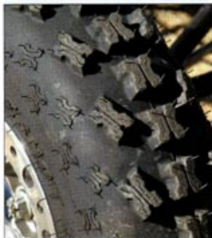
With revised sidewall knobs and a slimmer profile, the newest ITP Holeshot GNCC front tires measures out to 22x7-10 inches. This allows for a tall but quick-steering tire that tracks straight at high or low speed.
