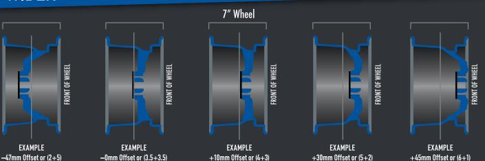
TRUE OFFSET: ET is the distance between the wheel mounting surface and the center line of the wheel. This measurement is commonly stamped in the back of your wheel. When ET is decreased in value the wheel will protrude further out. Example of ET measurements: -47mm/0mm/+5mm/+10mm/+30mm/+40mm
